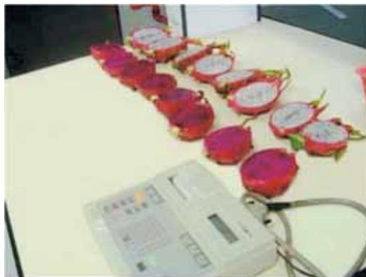
The hue angle correlates to the colour perceived by the human eye whereas the chroma provides a measure of the intensity of the colour. On-line colour sorting machines that function in a manner similar to laboratory equipment are widely used in commercial packing houses to grade citrus, mangoes, tomatoes and apples in accordance with their colour.
