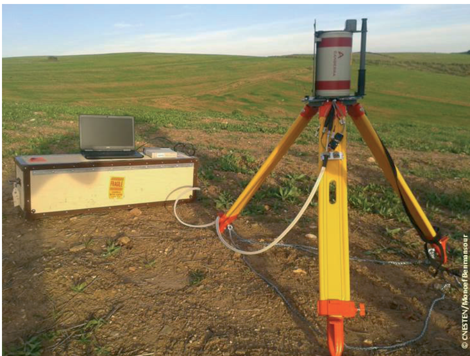
Figure 5.2. Portable gamma detector installed at selected study site (CNESTEN, Morocco).
