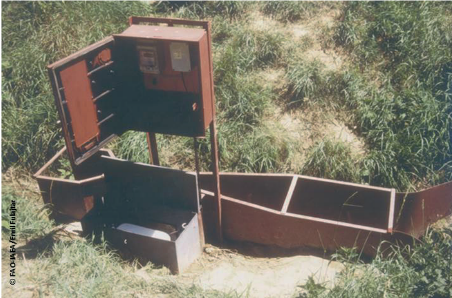
Figure 2.5. Example of Parshall flume used for measurements of suspended sediment (Lukacovce, Slovakia).
