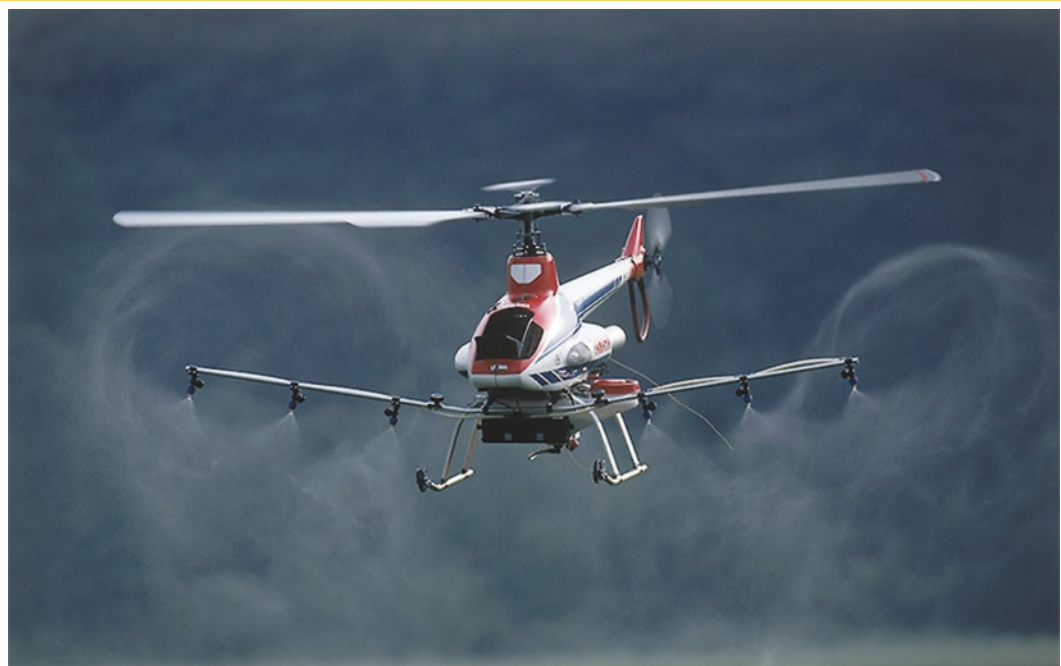
Figure F4. The R-50 uses the downwash from the main rotor to assist in spreading agrichemicals on the target area
