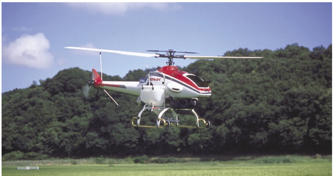
Figure F5. The RMAX Type II G comes with a high-precision GPS (2003)
