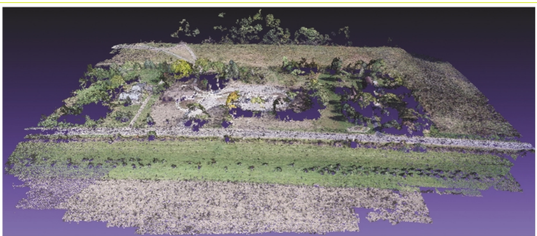
Figure D3. Three dimensional point cloud produced from thousands of images by ODM
