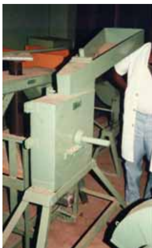
FIGURE 4 Locally made hammer mill and its typical construction
