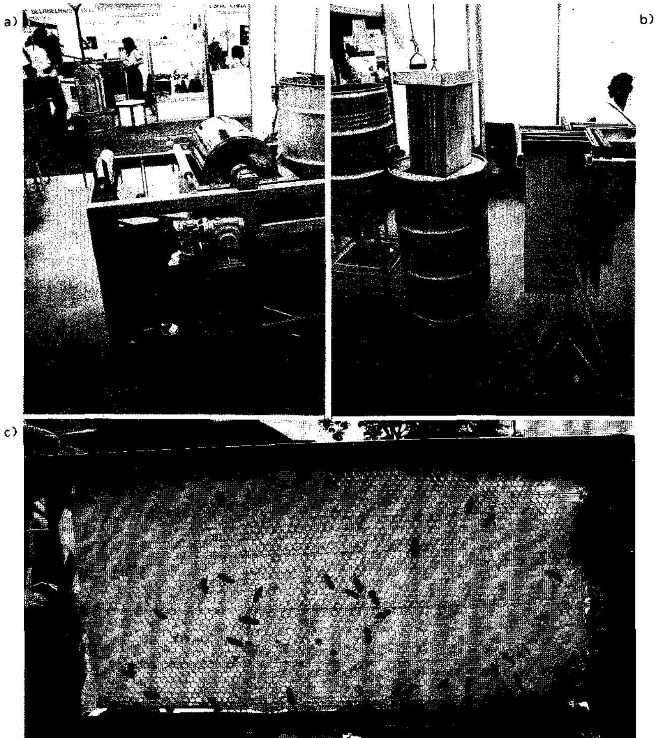
Figure 4.4: Top left: Medium size set up for the production of continuous wax sheets with a cooled drum rotating through a liquid wax bath. Top right: Rack and liquid wax bath for the production of multiple wax sheets by hand-dipping moist, wooden boards into the molten wax. Bottom: Wired frame with wired foundation sheet. All Langstroth and Dadant size frames should have at least four horizontal wires. Vertical wires can be embedded into the wax sheet by some manufacturers, but either of the wiring methods is usually sufficient.
