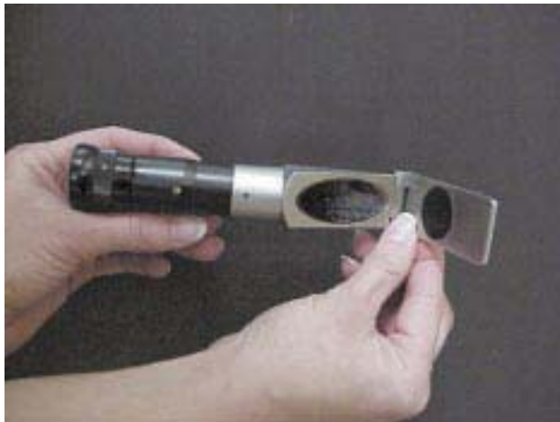
Figure 13.3: Hand and bench refractometers. For soluble solids ( ^{\circ} Brix) and specific gravity determinations.
