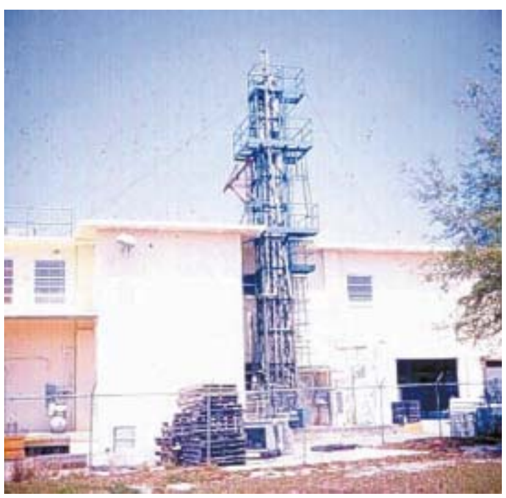
Figure 8.9: Essence recovery system schematic and commercial TASTE evaporator. Commercial units range to 20kL water/hr.
