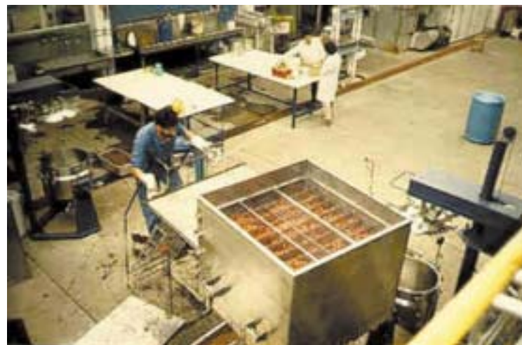
Figure 6.8a. and b: Steam extractors. Kitchen and pilot plant models.
