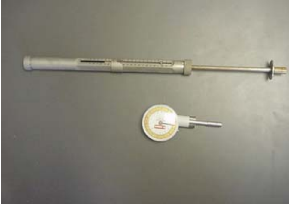
Figure 13.2: Penetrometer (Puncture pressure gauges). Penetration pressure is one indication of ripeness
