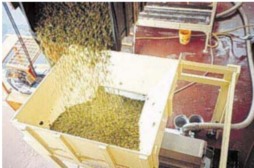
Figures 6.5a and 6.5b: Small and large fruit crushers. Capacity \sim 100 kg to 40 MT/hr.
