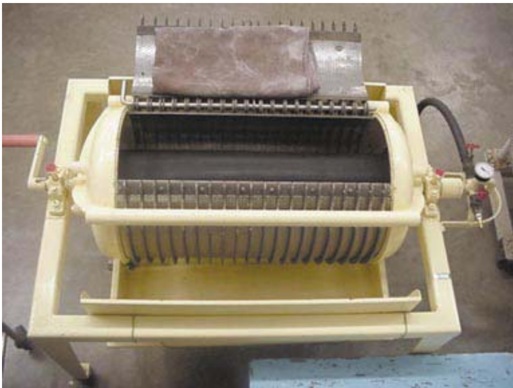
Figure 6.11: Bladder press, 100L capacity.
