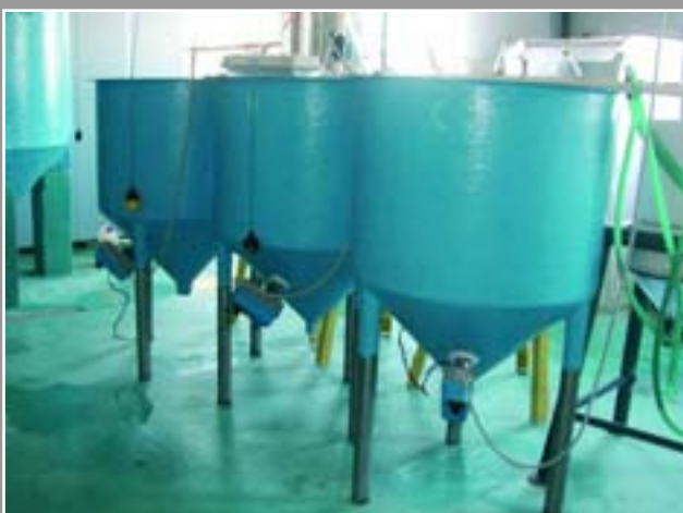
Fig. 83 - Tanks equipped with titanium heaters and thermostats
