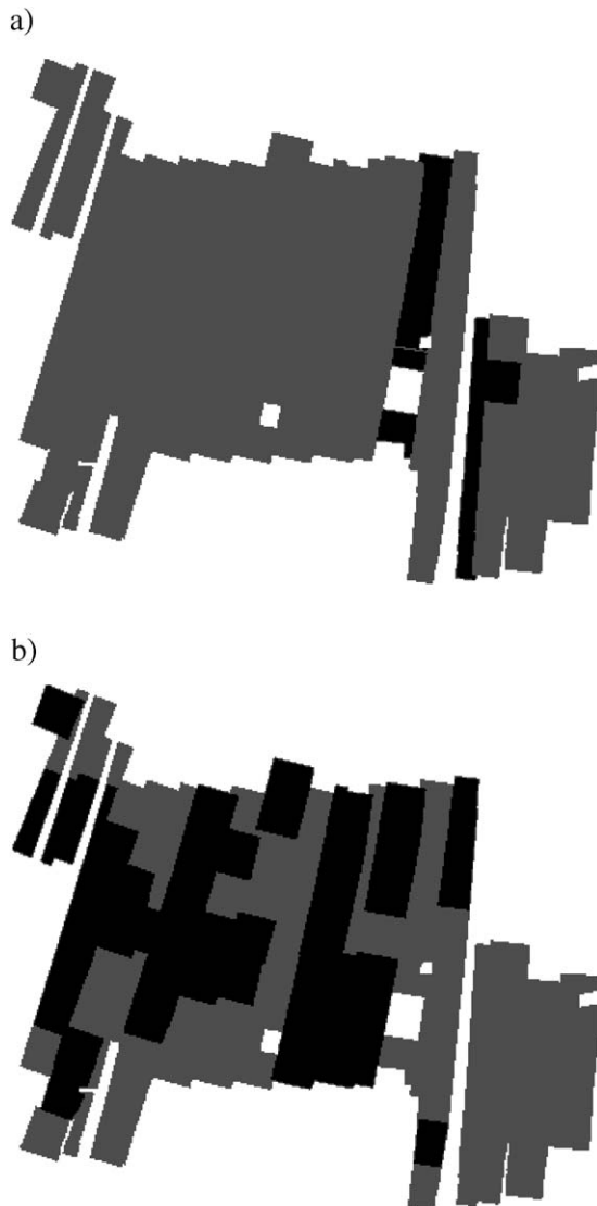
Fig. 3. Characteristics of the SIBERIA mosaic. (a) Relative coverage of fall 1997 (grey) and summer 1998 (black) ERS tandem data. (b) Relative coverage of GEC frames (grey: 74 of 122) and GTC frames (black: 48 of 122) in the mosaic.
