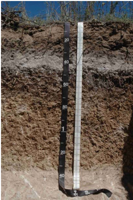
Left: Thaptoluvic Pisocalcic Solodic Planosol (Albic, Endohyposodic, Bathythaptopetroduric) Right: The excursion group standing in gypsum-rich sediments
