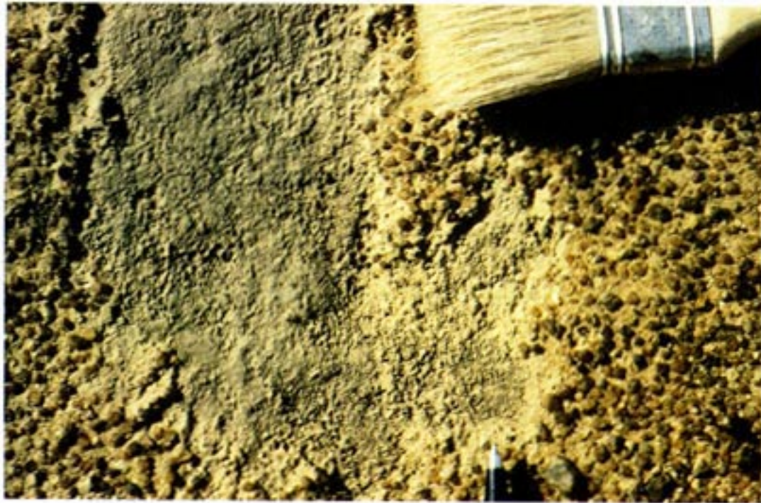
PLATE 9 Structural crust, three-layered sieving type, in Central Burkina Faso. Note the fine sand layer between the coarse sand layer and the fine particle layer
