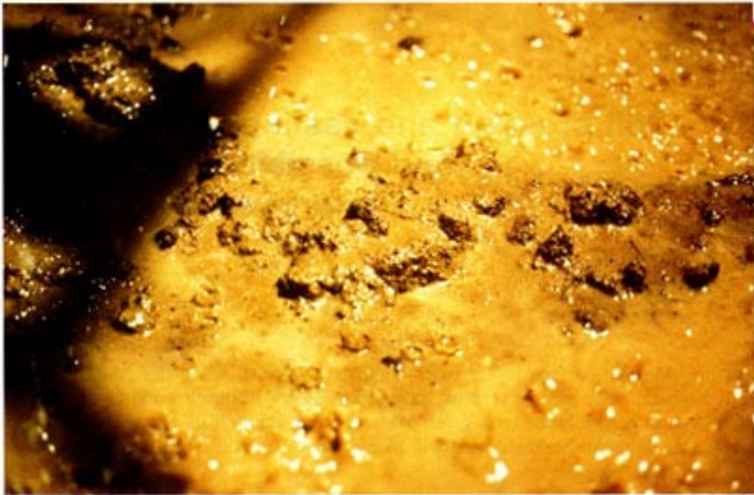
PLATE 7 Structural crust, slaking type, developed on a 'mound' in a clay loamy soil in northern Niger under simulated rainfall. Note the surface roughness. Depositional crusts are formed under the water layer
