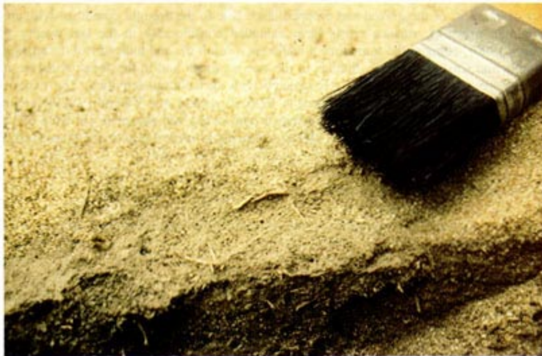
PLATE 8 Structural crust, two-layered sieving type, developed in a sandy soil in southern Côte d'Ivoire. Note the fine sand layer between the coarse sand layer and the fine particle layer
