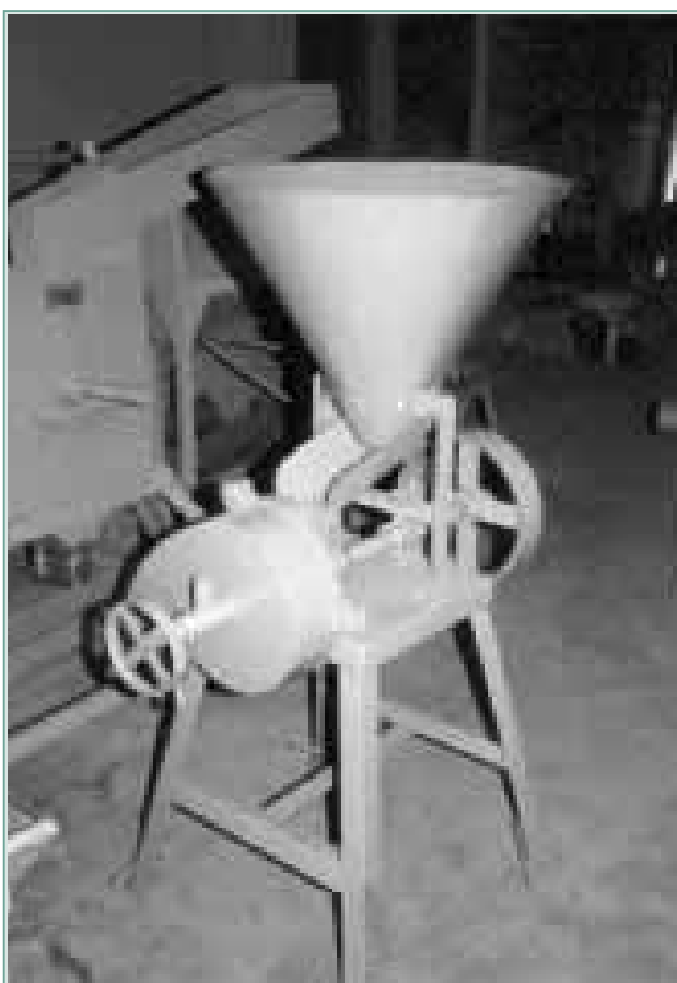
FIGURE 13 Locally made plate mill in Nigeria, used for wet and dry products.
