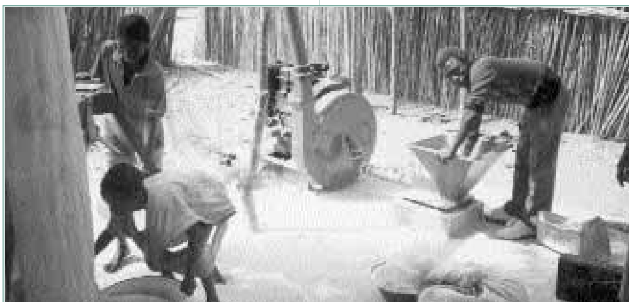
FIGURE 4 Hammer mill in the Congo driven by a diesel engine.
