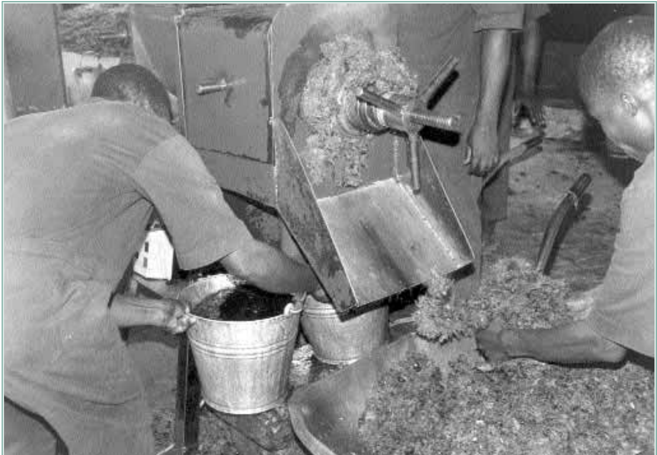
FIGURE 10 Larger-scale palm oil extraction in Benin using a screw press.
