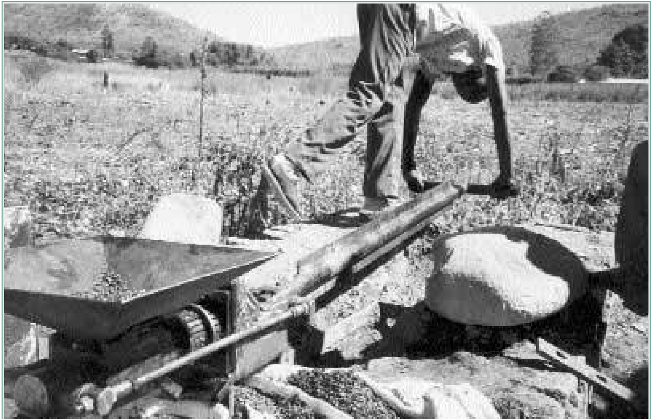
FIGURE 6 A Bielenberg lever press extracting oil from hybrid sunflower seeds in Zimbabwe.
