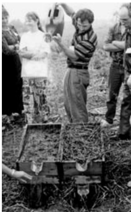
Demonstration of the impact of rain drops on bare and on mulch covered soil. Santa Catarina, Brazil
