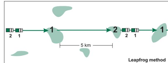
**Two vehicles:** nearly double the area can be covered when with two vehicles. The first vehicle surveys while the second vehicle drives ahead for about 5 km and then surveys. After the first vehicle finishes, it drives to meet the second vehicle. They both proceed together until the first vehicle stops to survey while the second vehicle continues for about another 5 km and stops for survey.
