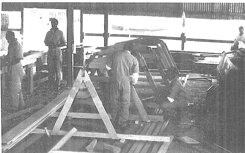
Fig. 2: The prefabricated frames for the 9.35 m canoe are erected on the building-jig.
