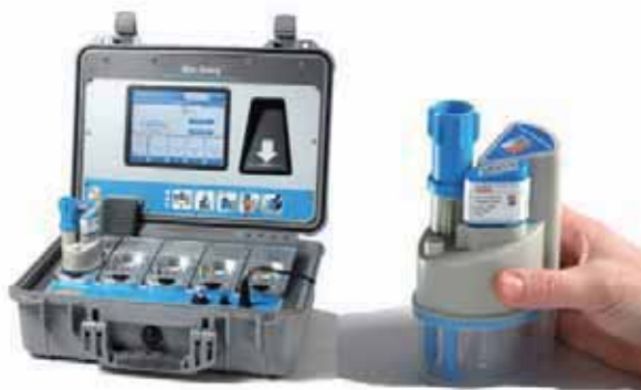
Figure 4. BioSeeq Portable Veterinary Diagnostic System. Pictured left: portable PCR instrument with five independent thermocyclers (running assay in far left thermocycler) with built-in communications including GPS, WiFi and Bluetooth technology. Picture right: disposable automated sample preparation unit (SPR) processes raw sample into PCR mixture allowing test to be conducted at pen-side.
