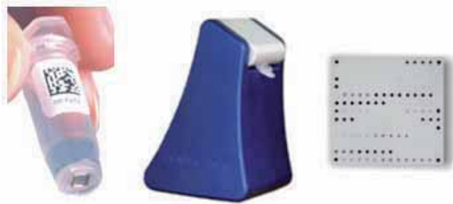
Figure 1. Clondiaq Chip technologies ArrayTube (AT) platform. From left to right: array tube (with probe array chip on the bottom of the tube), the ATR 03 reader (connected to a PC or laptop to run image acquisition and analysis), magnification of probe array chip (detection reaction consists of horseradish peroxidase and HRP-substrate tetramethylbenzidine which reacts to form a blue precipitate).
