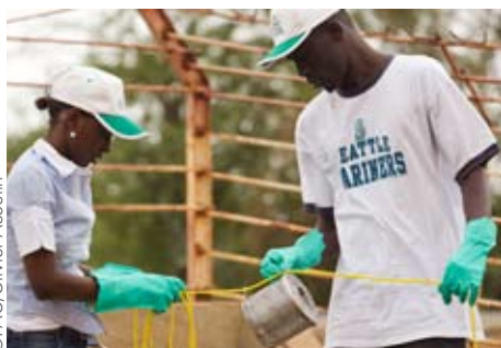
Senegalese technicians prepare a water filter to check for pesticide residues.
