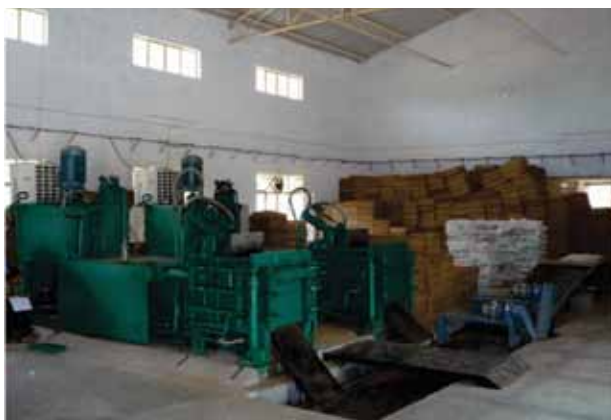
Photo 10. Densification machines based on the principle of hydraulic compression for making feed blocks
