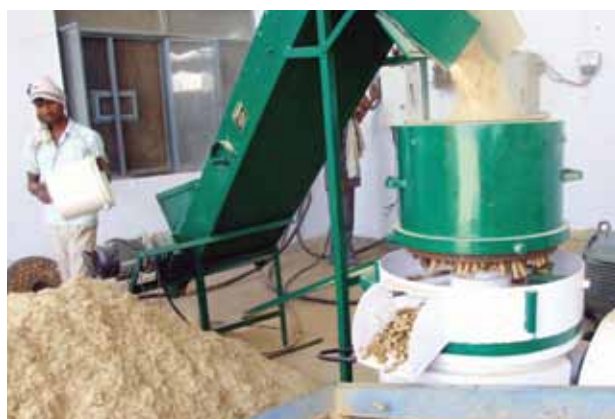
Photo 17. Pellet mill for enriched straw
