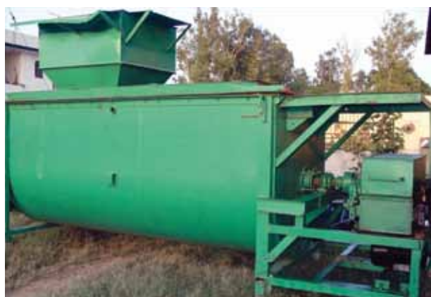
Photo 8. TMR mixer – single vat system for mixing straw and concentrate
