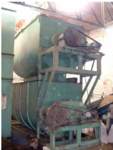
Photo 9. TMR mixer – twin vat system for mixing straw and concentrate
