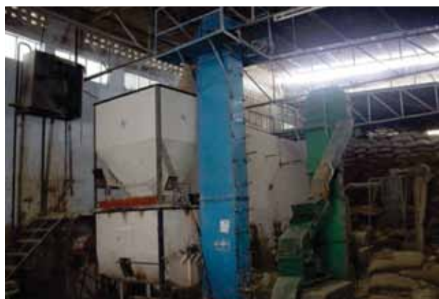
Photo 7. Grinder and mixer for making normal concentrate mixture
