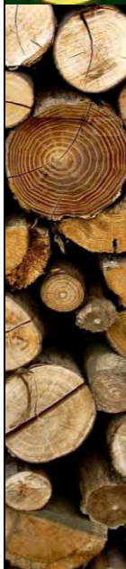
Eucalyptus log showing effects of release of stresses
