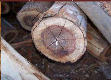
Eucalyptus log showing effects of release of stresses
