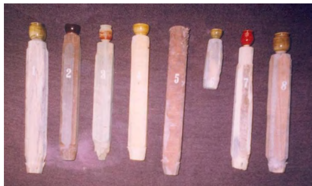
Trials by IWST with various alternative timbers (1.Cashew, 2.Chaplash, 3.Semul, 4.Ebony, 5.Red gum, 6.Rubber, 7.Subabul and 8. Bijasal)
