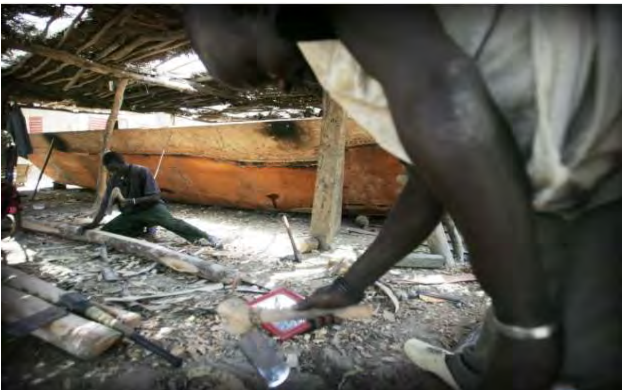
Boat builders in Nouhoun-Bozo shape wood to be used in the construction of large boats. While Nouhoun-Bozo is a very small village, they are a major supplier of boats to the large river port town of Mopti, about 75 km down river.
