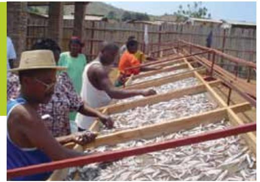
*With air circulation, the rack system reduces fish drying time from **three days to eight hours**.*
