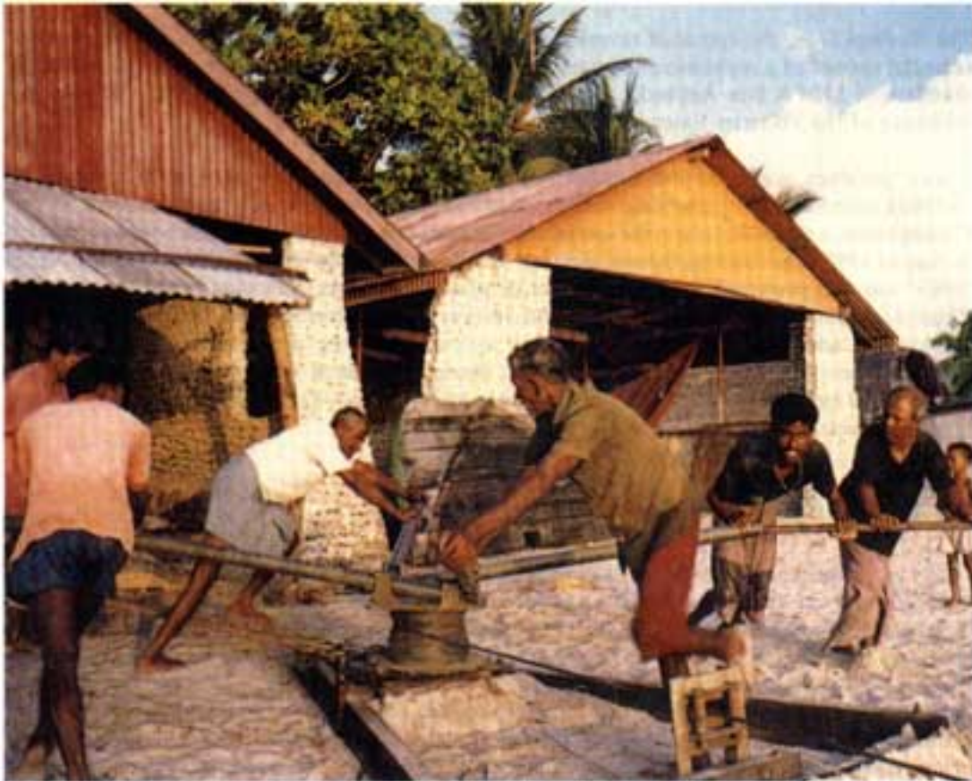
Among the manual boat hauling devices, the steel capstan was preferred.
