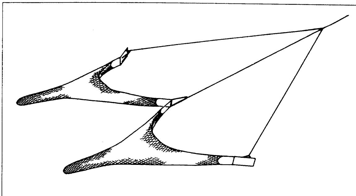
This rather particular gear comprises two identical trawl nets ('twin') working together, opened horizontally by a single pair of otter boards. Their inner wings are attached to a sledge towed simultaneously with the otter boards from a common warp. They are generally used for catching shrimp (four trawls at the same time).
