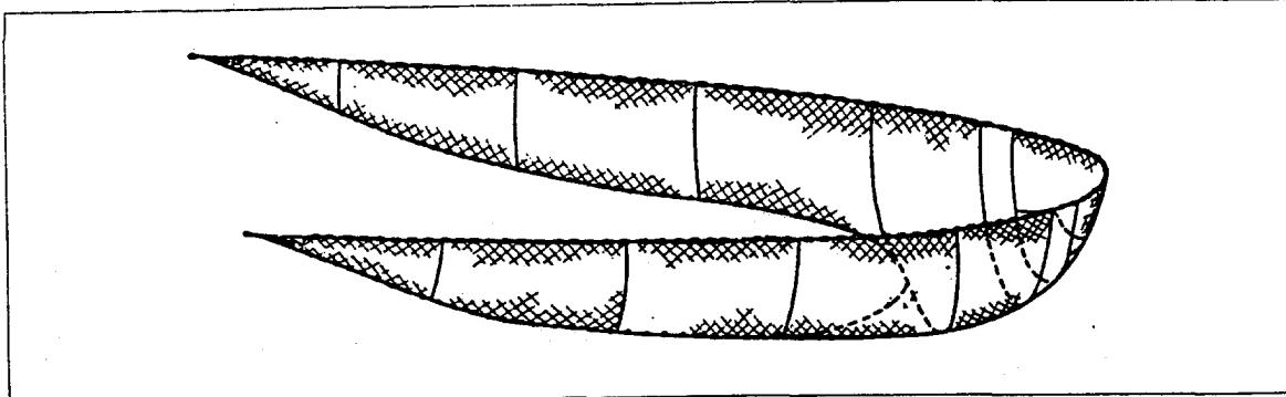
The lampara net is the type most representative of this category. Its particular design, with the central bunt in the form of a spoon and two lateral wings, makes it possible to retain the shoal of fish when the two wings are hauled up at the same time.
