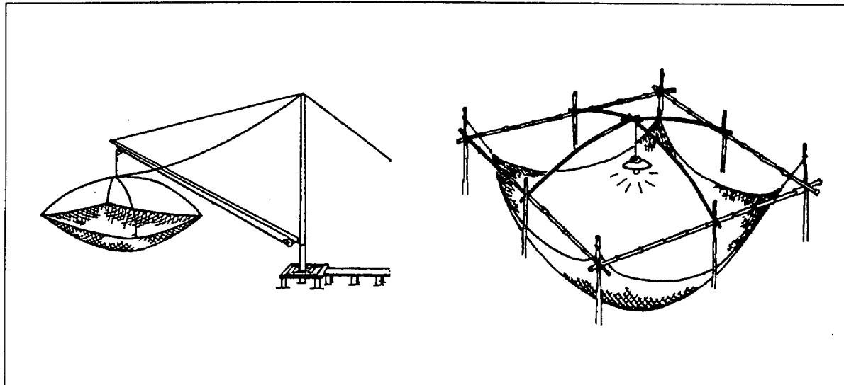
These lift nets are usually operated from stationary installations situated along the shore, the lifting system sometimes being mechanized.
