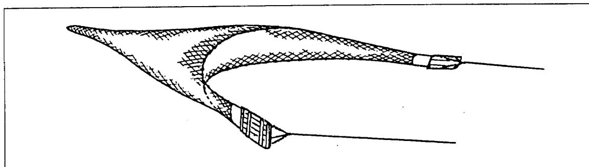
These are trawls towed by a single boat; their horizontal opening is obtained by otter boards, relatively heavy and equipped with a steel sole designed for good contact with the ground<sup>1</sup>.
