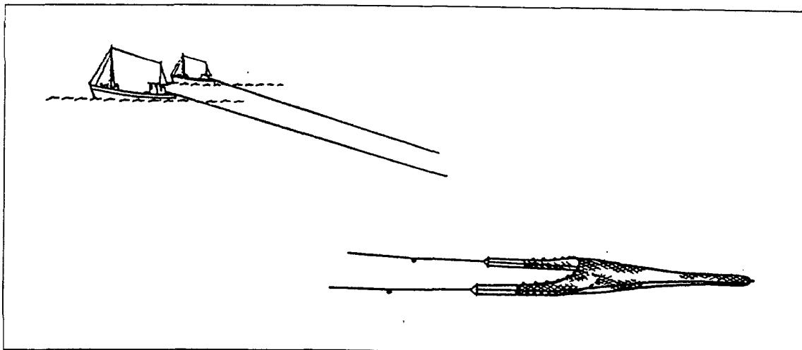
These trawls are towed by two boats at the same time, the distance between the boats ensuring the horizontal opening of the net.
