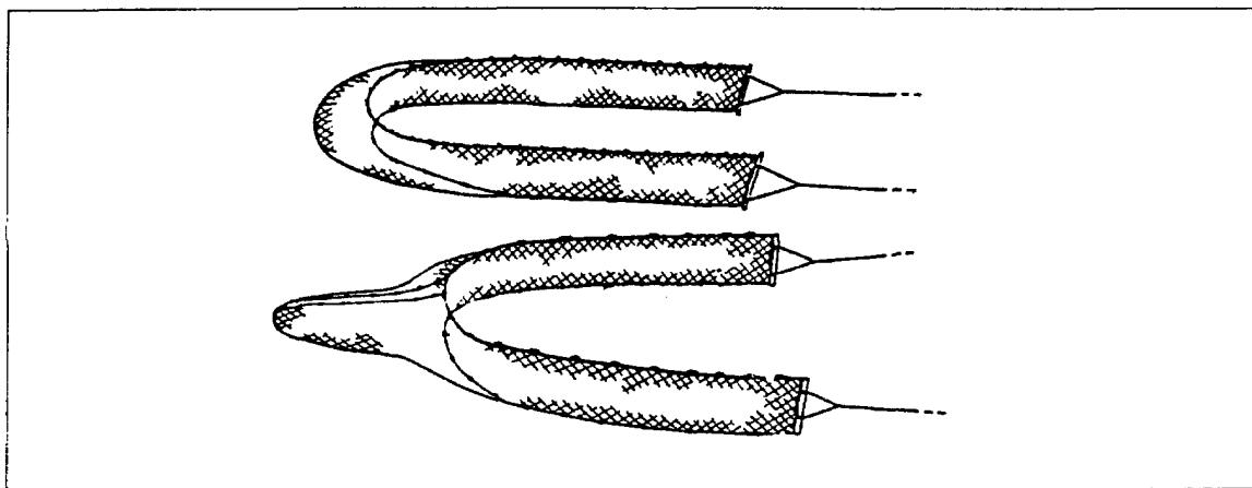
This category comprises the seines operated from land, which are generally used in shallow waters, near the shore; the bottom and surface act as natural barriers which prevent
