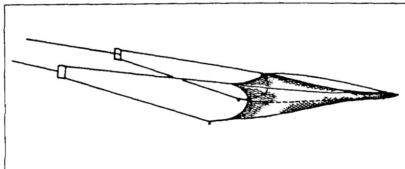
These trawls are towed by a single boat. The horizontal opening of the net is controlled by otter boards, usually of a hydrodynamic shape, which normally do not touch the ground.
