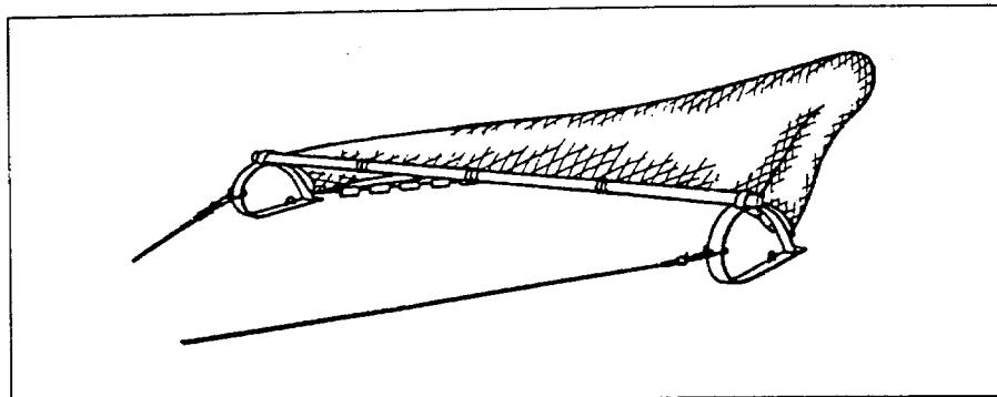
In these trawls, the horizontal opening of the net is provided by a beam, made of wood or metal, which may be 10 m long or more. Beam trawls are used mainly for flatfish and shrimp fishing<sup>1</sup>.
