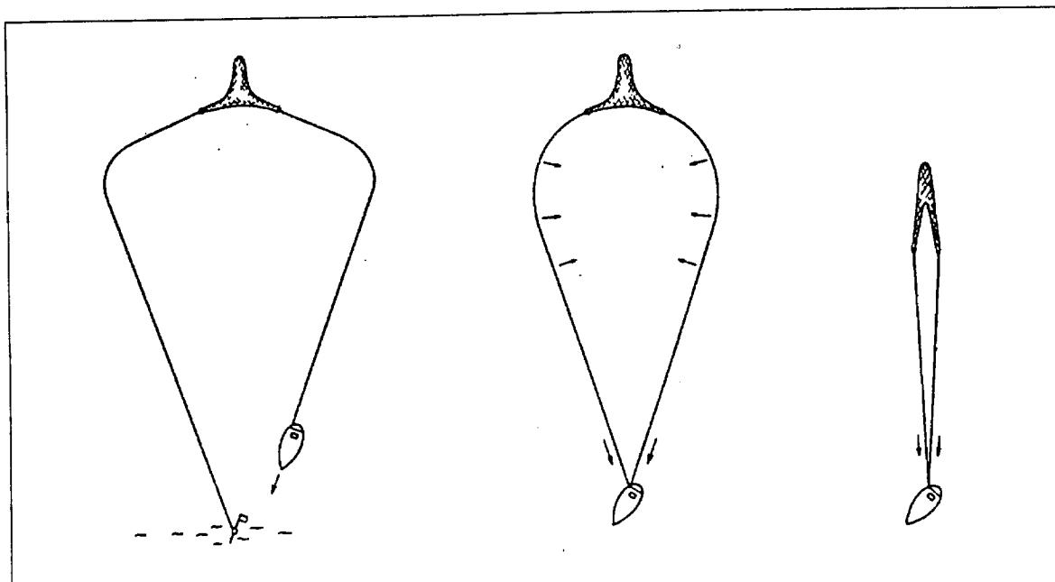
The type most representative of this category is the Danish seine. The design of these nets, consisting of two wings, a body and a bag, is similar in many ways to that of trawls.
