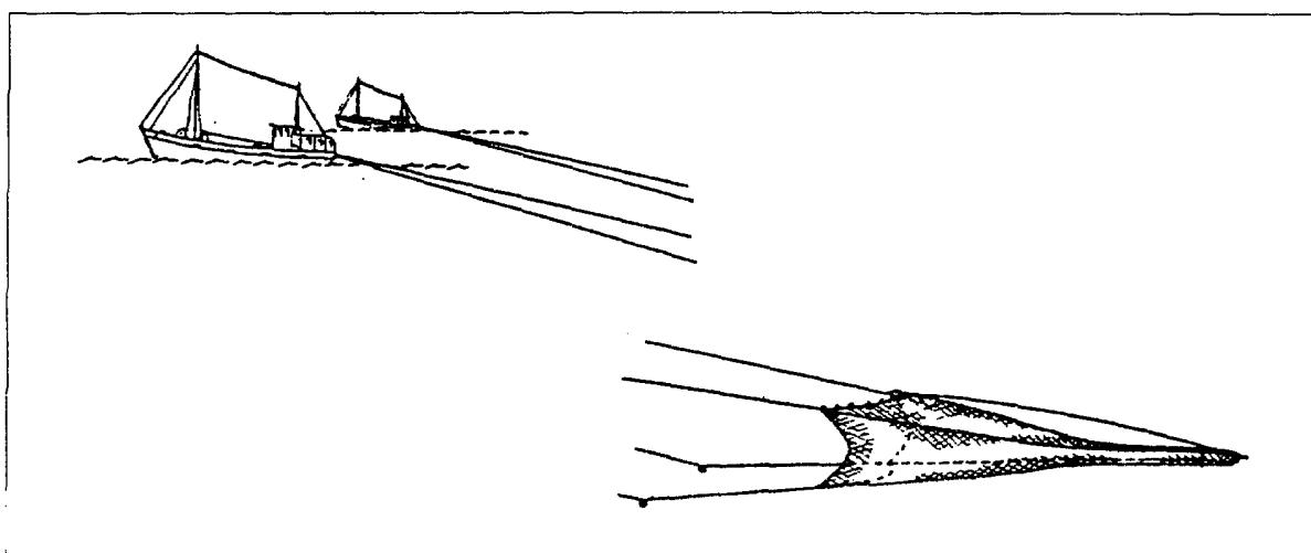
Towed by two boats, thus ensuring the horizontal opening of the net, these nets are designed and rigged to work in midwater. Surface trawls are also included in this category.
