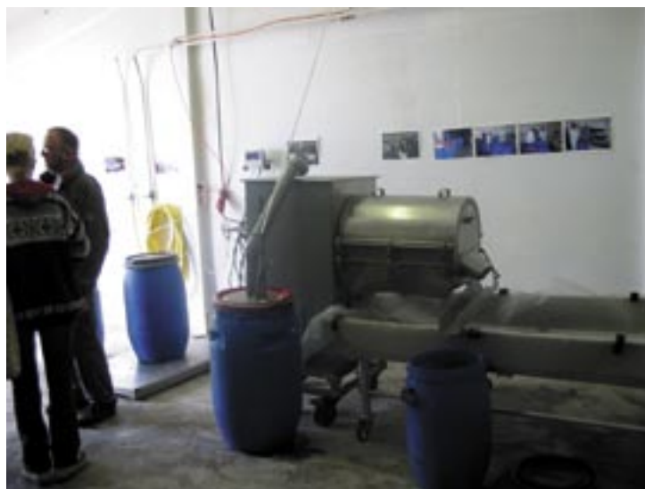
Screening machine at a demonstration in Drangsnæs, Iceland, 2003. Compressed air is used to pump the roes from the landing containers to the screening machine
