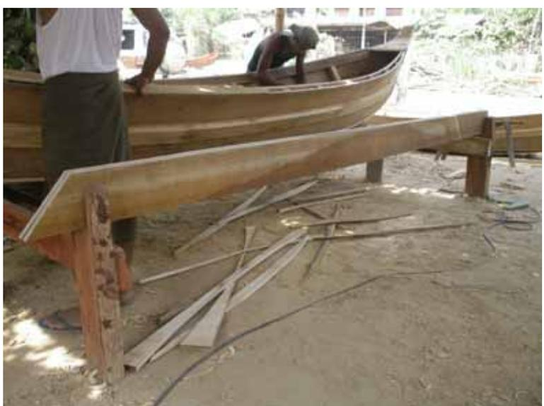
A person is working on the lower side planks of a boat hull. The planks are clamped together and are being shaped. The boat is resting on a wooden stand. The background shows an outdoor workshop setting with other boats and structures.                        |
