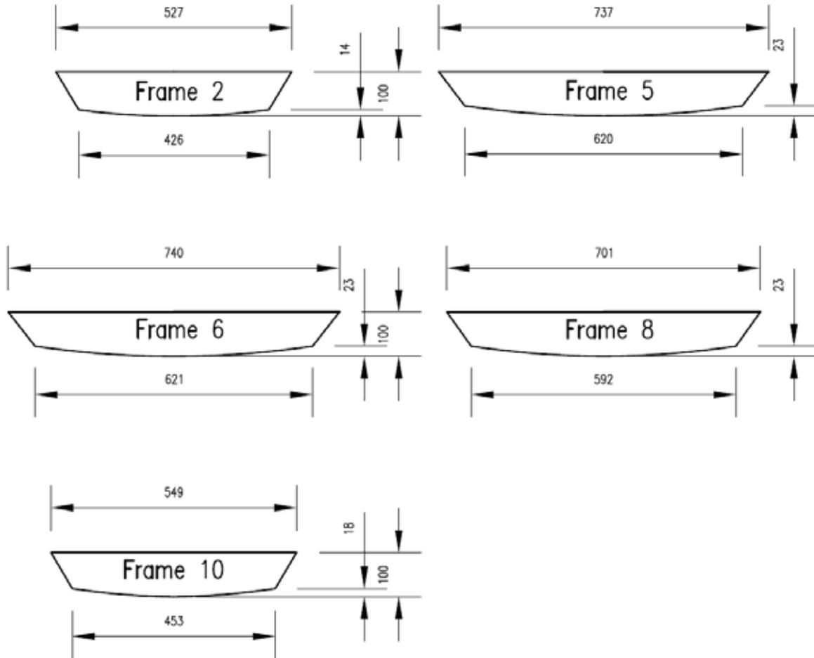
Note: The dimensions for floors at other frame positions may be determined once stem and transom are fitted (see step 19).
