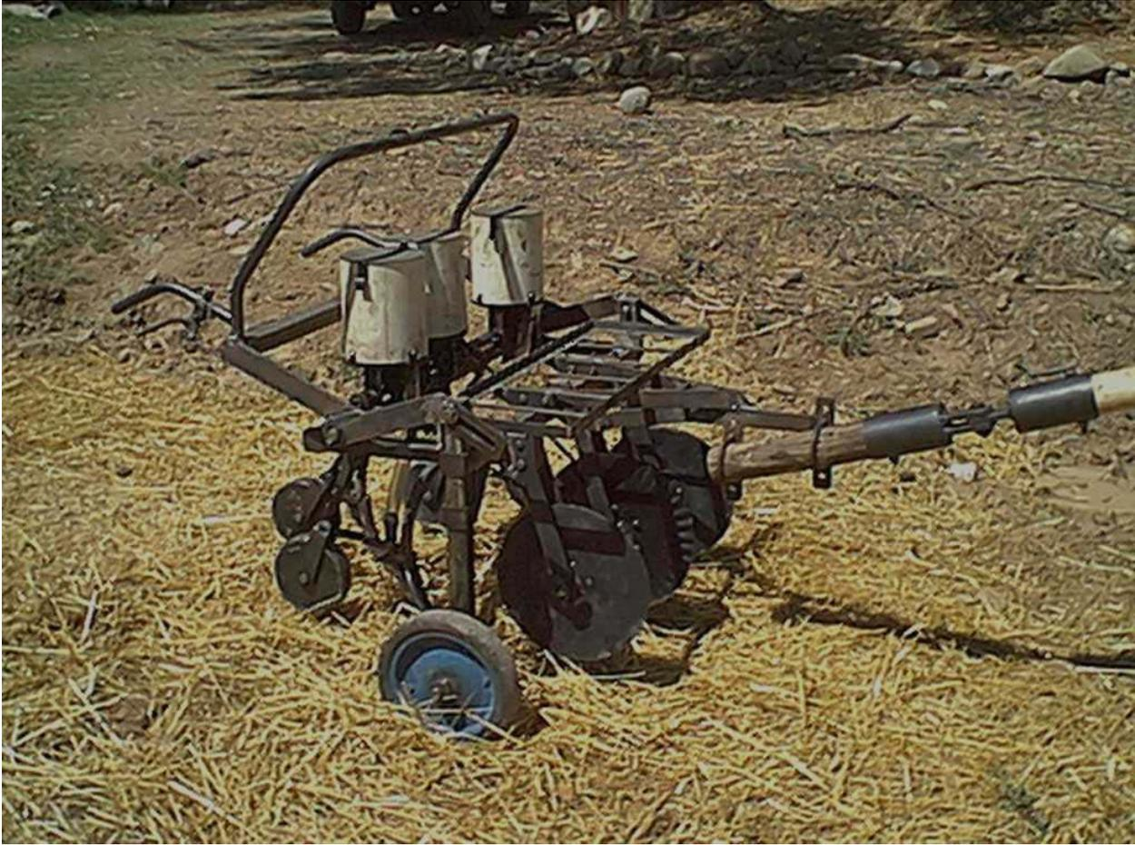
Figure 1. Conformation of the seeder for direct seeding using the horizontal plate seed metering system, and equipped with the articulated draw-pole connector.
