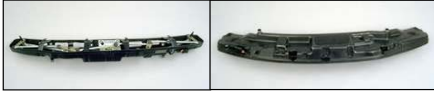
figure 2.3: Single step manufacturing. Left: “old” multiple parts car dashboard. Right: Integrated “new” composite design of the same dashboard
