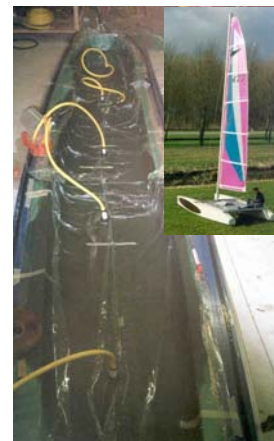
figure 4.3: A flax –reinforced catamaran hull
