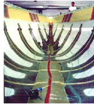
figure 2.10: Vacuum injection of a boat hull
