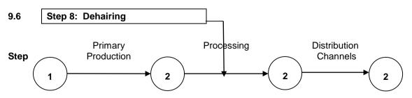
29.32. This is the point in the process where the hair is removed from the animal. During dehairing manure is pressed out of the rectum and accumulation of manure and growth of *Salmonella* in the equipment can occur. Among the operations carried out in the unclean area, dehairing and singeing/flaming operations
