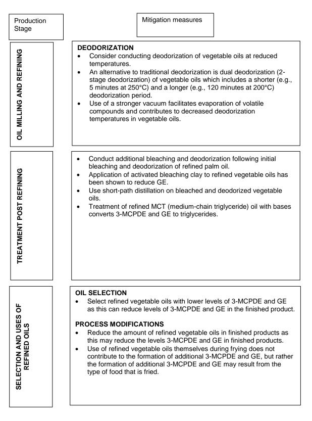
\*Although this document addresses both methods in use by industry and those in their experimental stages, only those methods that are used in industrial applications are shown in the diagram.
