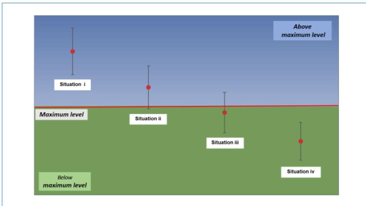
Figure 1: Taking into account the expanded measurement uncertainty in the comparison of test results with a Maximum Level. For each situation, the red point represents an individual test result and the vertical bar represents the associated measurement uncertainty interval.
