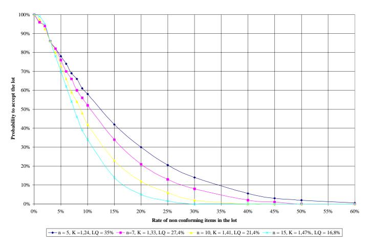
OC curve of a variable sampling plan, AQL = 2,5%, n between 5 and 15
