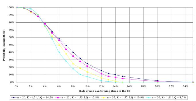
OC curve of a variable sampling plan, s method, AQL = 2,5%, n between 20 and 50
