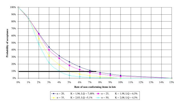
OC Curve, variable sampling plan, method s, AQL = 0,65 %, n = 20 to 50
