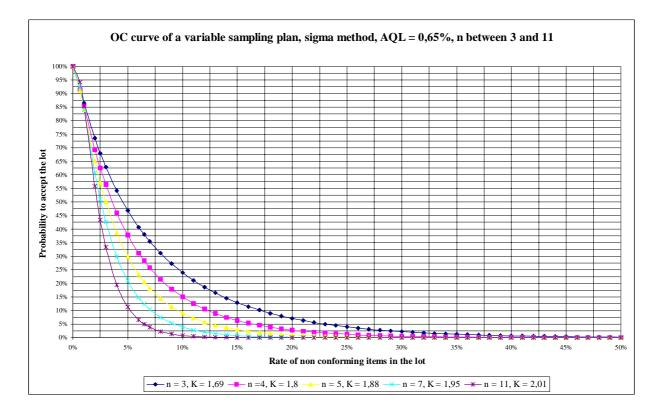
Figure 13: OC curve, variable sampling plan,  $\sigma$ -method, AQL = 0,65 %, n = 3 to 11
