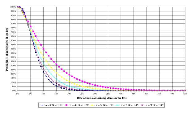
OC curve : variable sampling plan, sigma method, AQL = 2,5%, n between 3and 9
