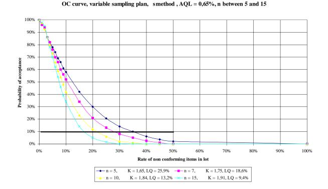
Figure 9: OC curve, variable sampling plan, s-method, AQL = 0,65 %, n = 5 to 15
