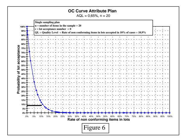
Figure 6: OC curve, attribute sampling plan, AQL = 0,65 %
