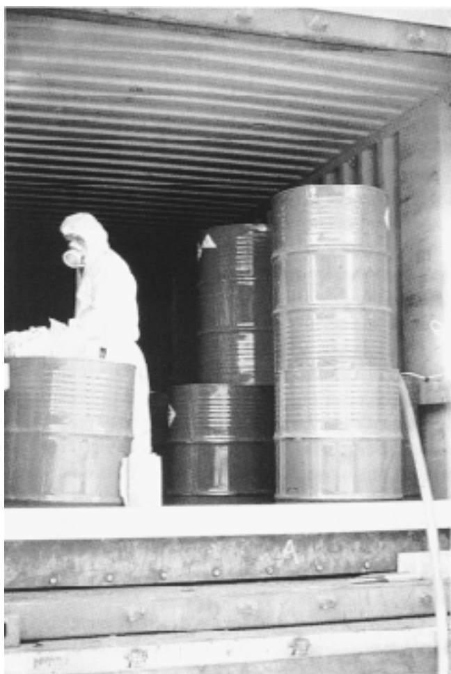
FIGURE 7 One of the steps necessary in decanting, repackaging and transporting obsolete, unwanted and banned pesticides in an affected country. The disposal process can be hazardous when appropriate care and precautions are not taken
