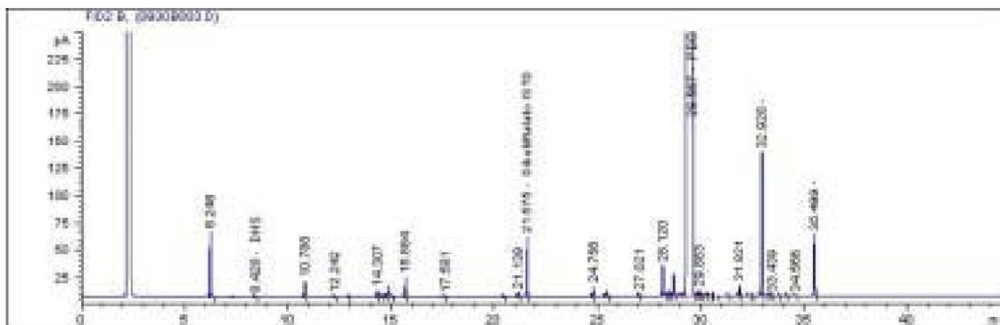
If the peaks retention time is not within the quoted window, the oven temperature or the column head pressure may need to be checked or slightly adjusted.
