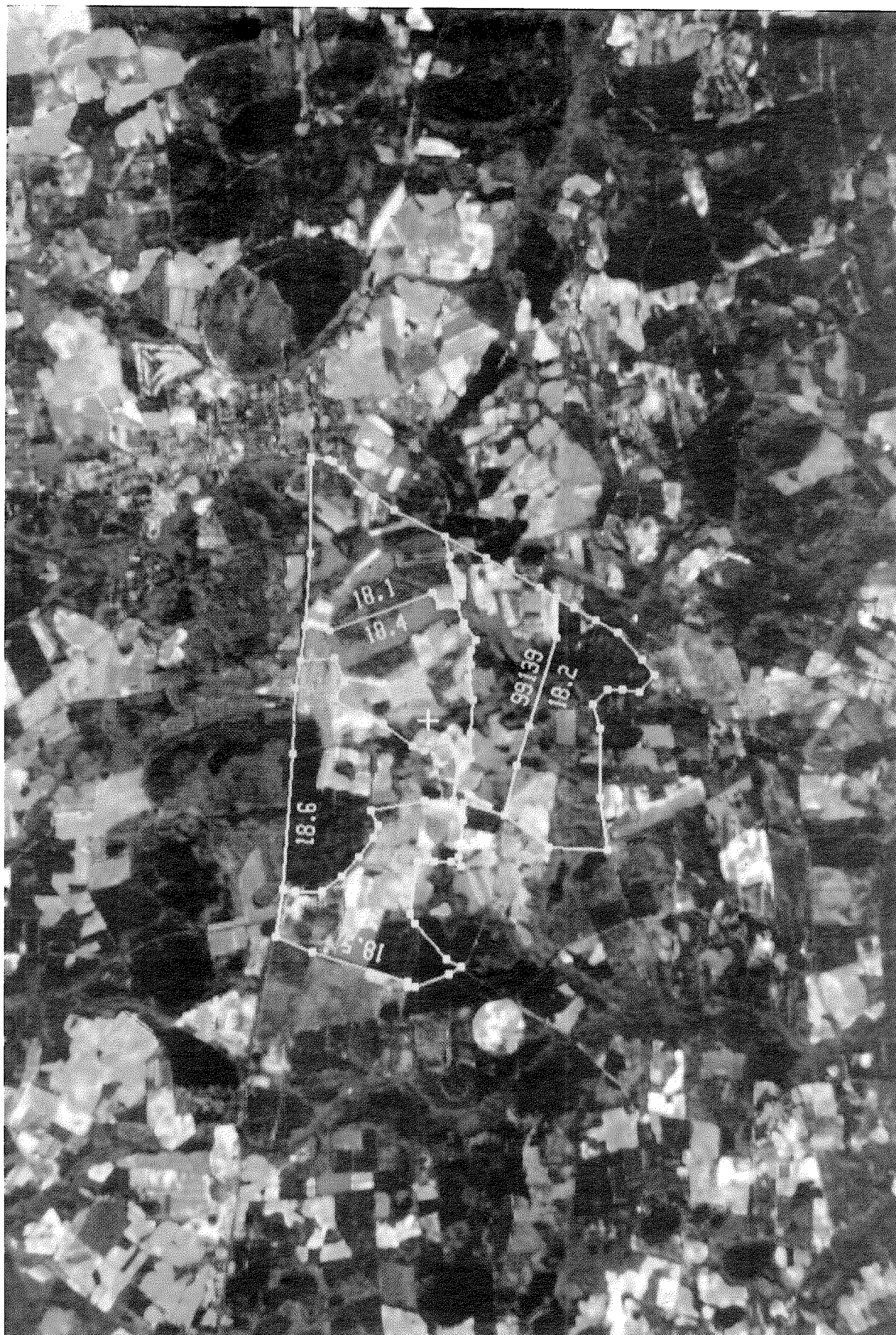
Figure 5. A TM/LANDSAT scene with a PSU broken up into segments.
