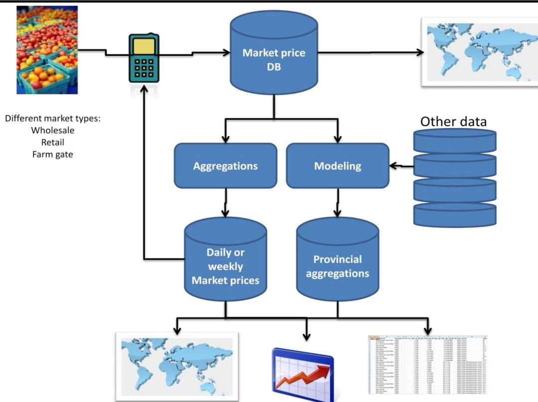
Data is collected from markets using ad-hoc forms built in the smartphone application. The smartphone send data to the database that displays them on a map on real-time basis. The processing aspect involves a) aggregations to derive daily weekly and monthly prices and b) modeling to estimate market price data at provincial level by combining market price data with other relevant information from other data sources.
