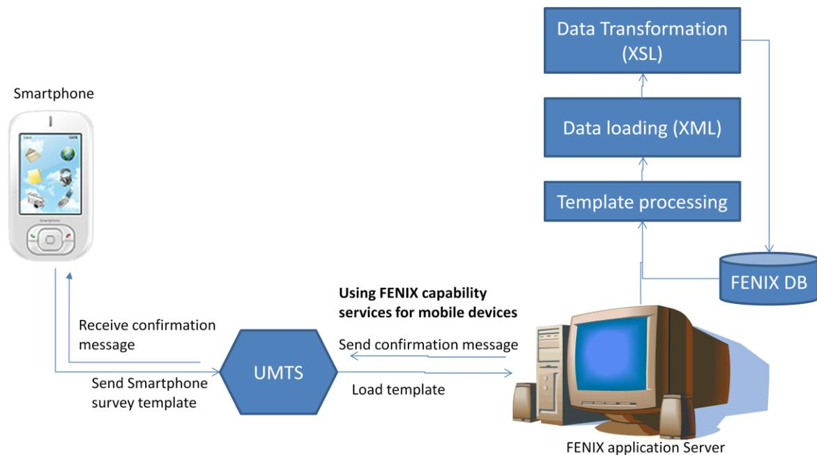
Data collected in the field using the system describes above are stored in a temporary database, where data is checked and validated before it is sent to the production database and published.
