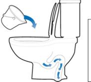
Flush toilets have a tank and pour flush have no tanks. But flush toilet with a tank can act a pour flush but not the other way around.
