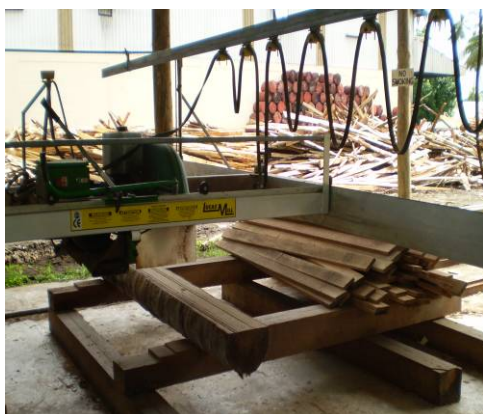
Figure 13. Lucas Circular sawmill, powered by diesel engine and electric motor (Fiji)
