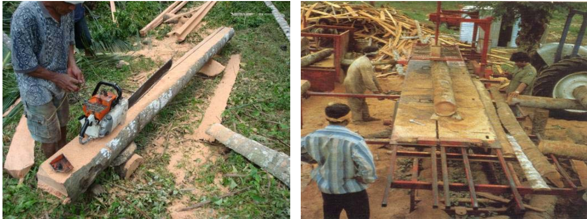
Figure 14. Using chainsaws is popular in rural areas in small scale operations (left). But in large scale operations, bandsaws or circular mills, like the Varteg sawmill in Vaitele, Western Samoa (right), are used
