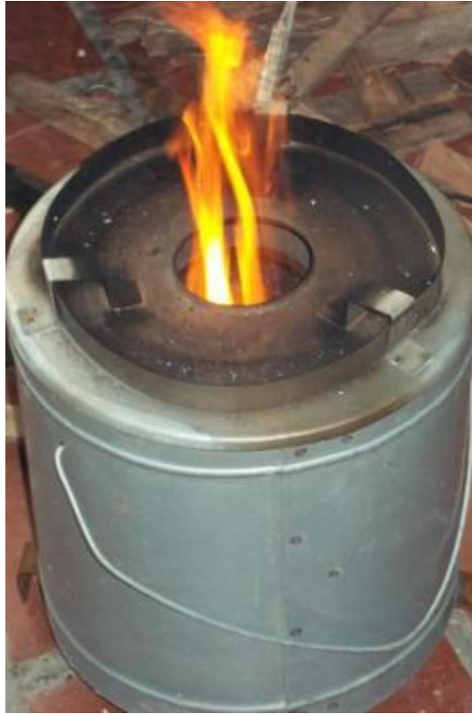
Stove for cooking and making biochar, Hanoi
