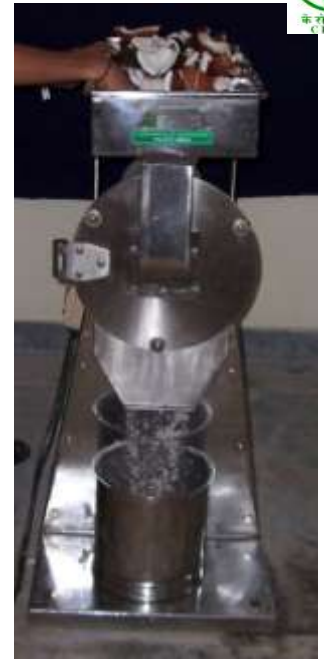
Coconut Grating Machine Capacity: 200 nuts/minute
