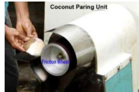
Coconut Testa Remover Capacity: 45 nuts/hr
