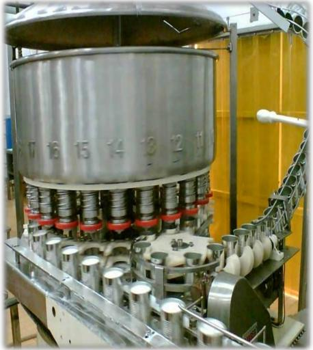
The process of packing coconut milk in the cans
