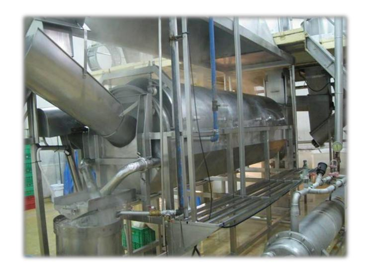
We soak coconut meat in a blanching machine at the temperature of 75 c. or higher for 1.5 minutes.
