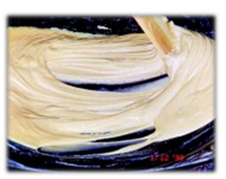
Stir with stirring device, then bring the pan down from the furnace
