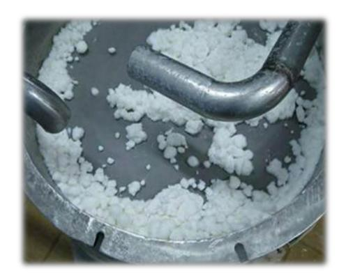
We separate coconut milk and coconut pulp using the vibration filter.
