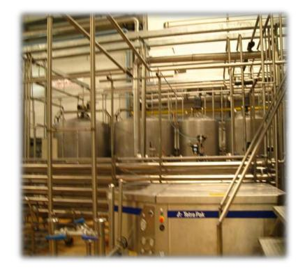
Process for homogeneous coconut milk. that before product through this unit system must be pass stainless steel sieve filter 60 mesh.
