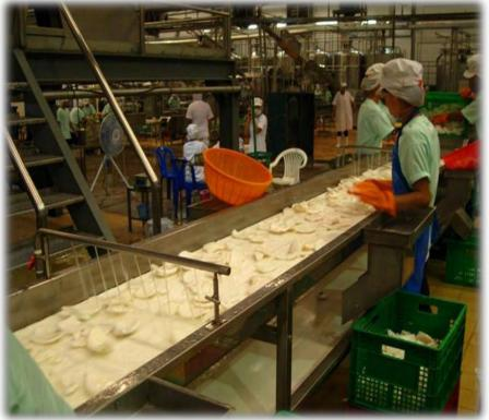
We double check the quality of the coconut meat again while coconut meat is being washed and cleaned with softened water at the temperature of 25 - 35 c.
