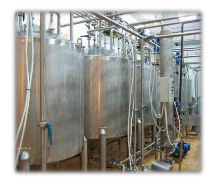
For the process of ingredients mixing, we add all ingredients into coconut milk extract to adjust the taste and its appearance. One mixing tank is for one formula.
