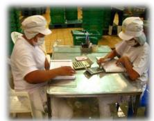
The process of Closing the lid by seamer and inspection work in process by visual check and tear down.
