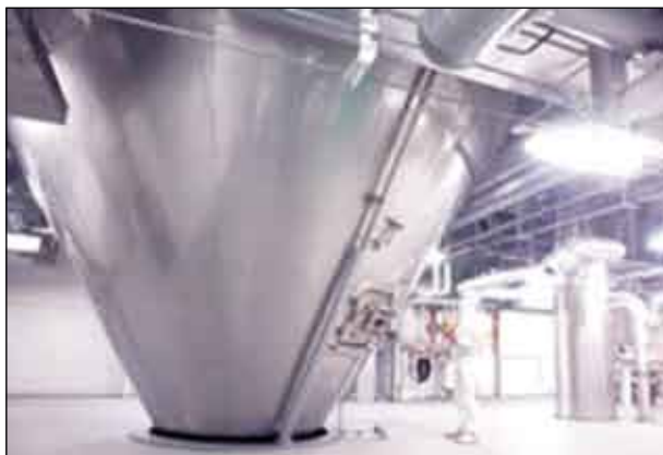
5(d) Medicinal components concentrated by spray driers.
