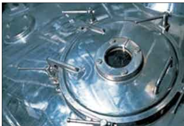
5(c) Medicinal components in crude drugs extracted in a large tank and residues are removed by centrifugation.
