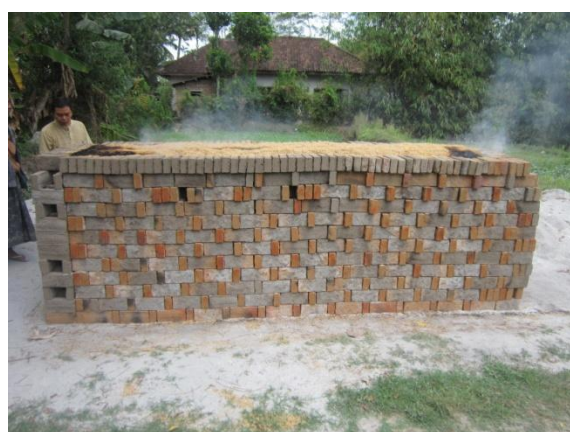
Figure 9: Kiln used for drying tobacco using palm kernel shells
