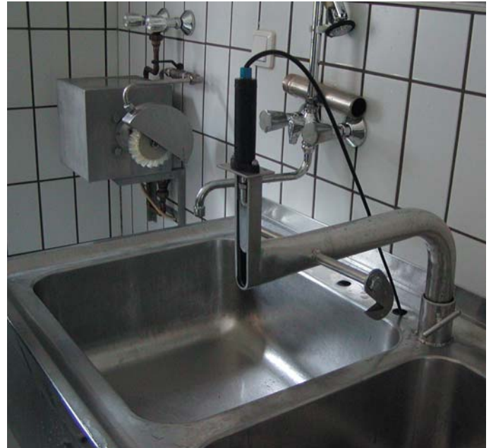
Figure 2: A simple but highly sufficient place to clean fish (above left). Knife to cut the belly and vacuum gutting device fixed together near to the wheel brush to clean the fish from inside (above right and left below)
