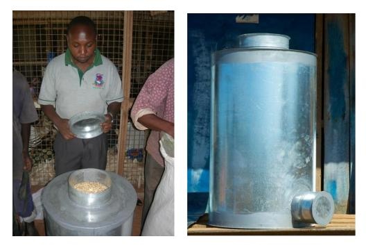
Figure 9: Metal grain silos for small scale storage
