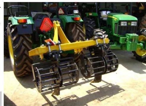
**AFGRI 2-tined ripper with clod-crushing cage wheels designed for contract ripping**
