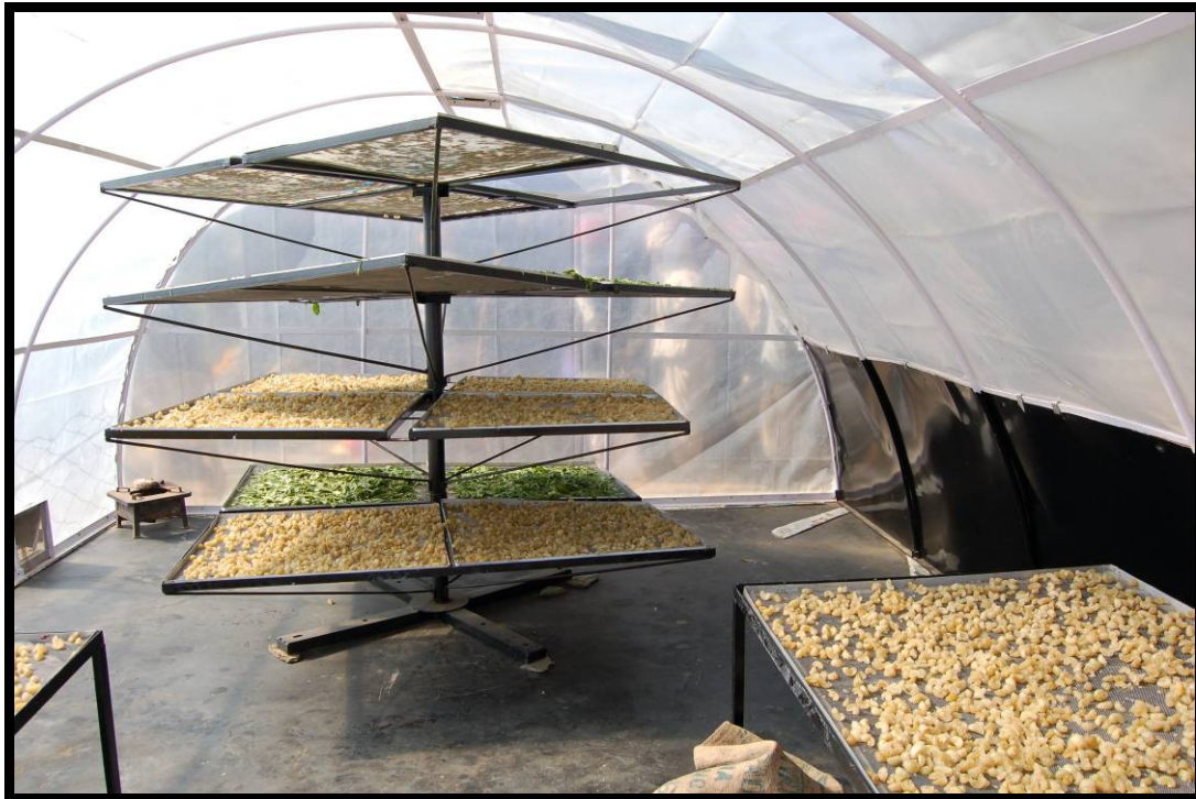
Fig 2 :Drying conditions under the tunnel drier
