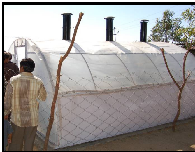
Fig 1: Locally made solar tunnel drier
