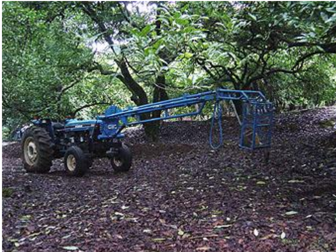
Figure 22 Harvesting machine to collect avocado
