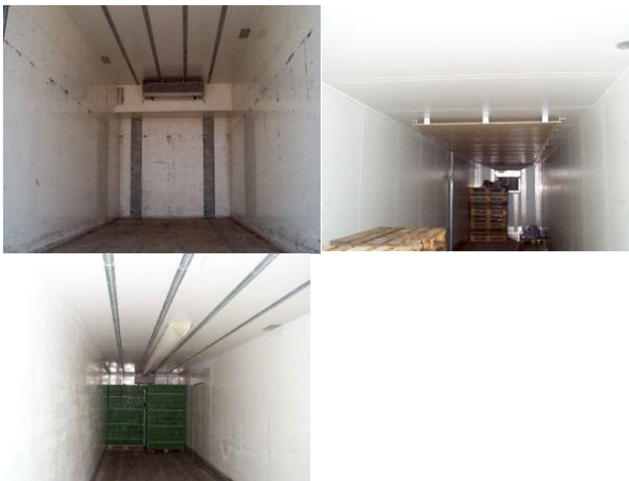
Figure 27. Air distribution systems in truck trailers for table grapes.
