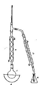
Apparatus for hydrolysis
