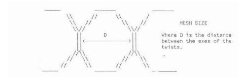
Gabions shall be of the types and sizes shown on the Drawings. The cages shall be constructed from mild steel wire complying with BS 1052, "Specification for mild steel wire for general engineering purposes", galvanised in accordance with BS 443, "Specification for testing zinc coatings on steel wire and for quality requirements". Wire used for the formation of the mesh panel will have a diameter of 3.0 mm.
