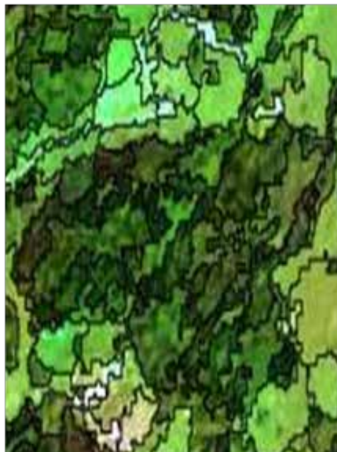
Fig. 6: Segmentation of forest area based on IRS-1D and Landsat TM fused image (source: Ivits et al. 2004)
