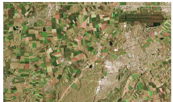
Fig. 8: Colour-coded TerraSAR image north of Munich. Data take 26. June und 7. July 2007, 5:26 UTC, resolution: 3 m, mode: Stripmap, polarisation: VV und HH (source: DLR, Germany)
